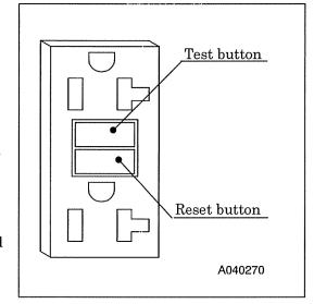
IF THE GFCI CANNOT BE RESET: The GFCI is faulty. Contact your nearest dealer. IF THE GFCI RESETS PROPERLY: Check the appliance or the power cord.
